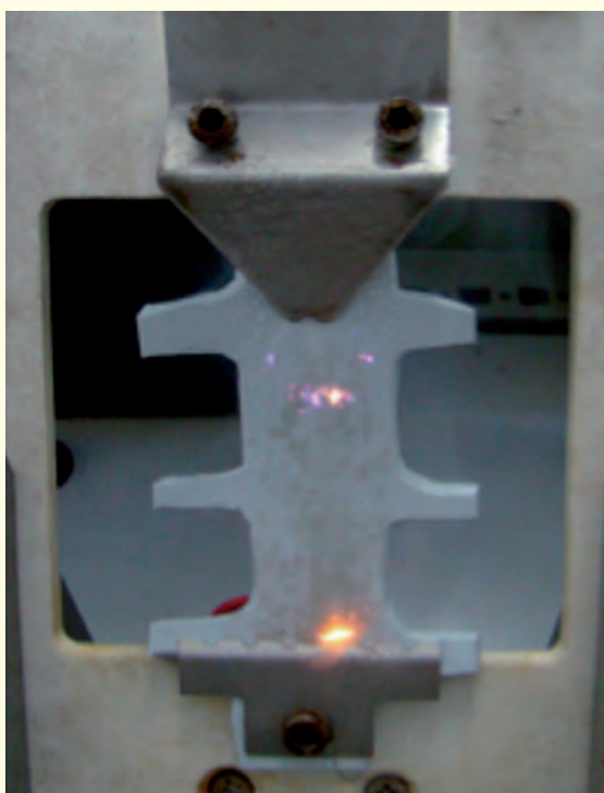
Inclined plane test with a specimen cut from an insulator housing
